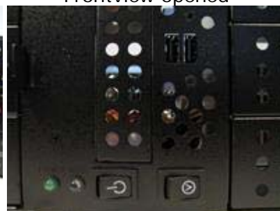
USB connectors, Power / HDD LED's, On -/Off switch, Resetbutton.
