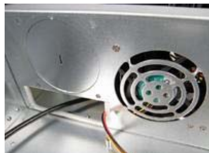
80mm fanpreparation on top of the protected cable hole, 80mm fan.
