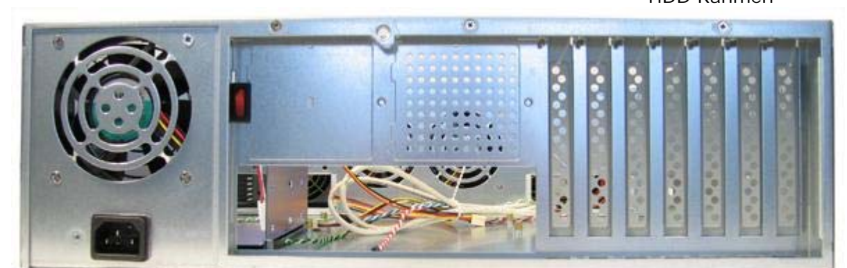
Backside: 1x 80mm Fan, Power connector, I/O shield area, on top 2x 60mm fan preparation, PCI-slots
