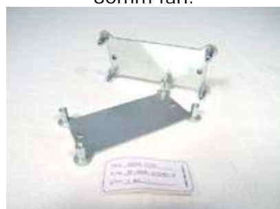
Dual Xeon fan mounting plates
